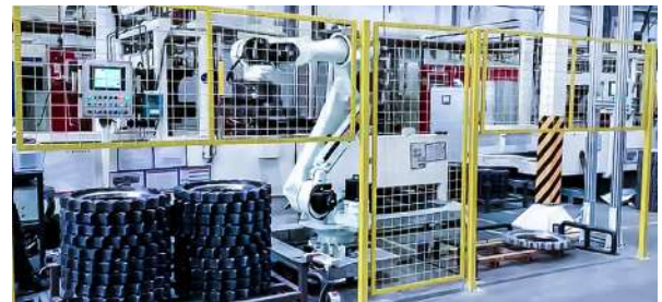
Vision-Guided Machine Tending of Drive Gears
