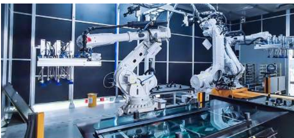
Vision-Guided Window Glass Gluing
