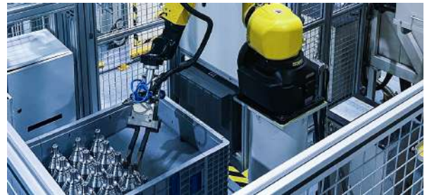
Vision-Guided Bin Picking of CV Joints
