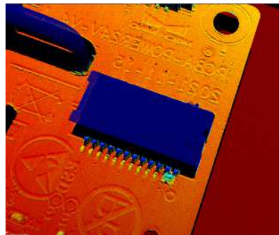
Chip pins (submillimeter welding defects)
