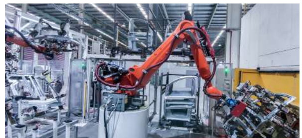
Vision-Guided Car Door Inner Panel Picking
